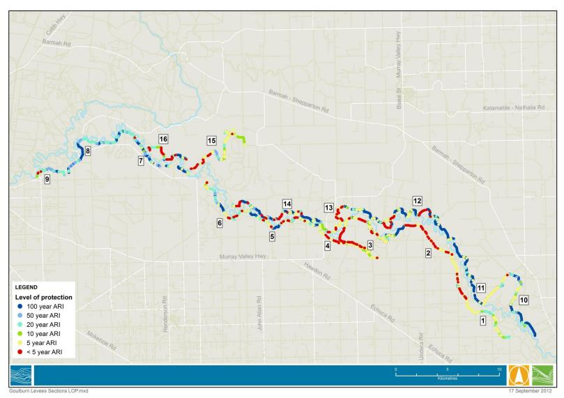
Figure 3-9 Map of level of protection of Goulburn River levees (Due to the scale of mapping, points overlap with the lowest LOP taking precedence)
