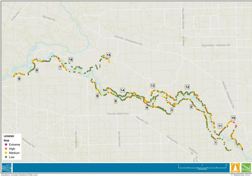
Figure 4-4 Points of weakness risk mapping for the Goulburn River levees. (Due to the scale of mapping, points overlap with the highest risk taking precedence)
