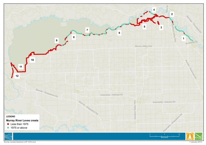
Figure 3-8 Map of Murray River levees crest levels compared to 1975 levels (Due to the scale of mapping, points overlap with < 1975 level taking precedence)
