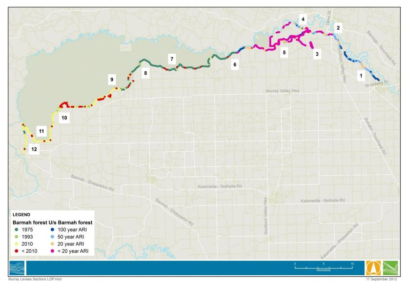
Figure 3-7 Map of level of protection of Murray River levees (Due to the scale of mapping, points overlap with the lowest LOP taking precedence)
