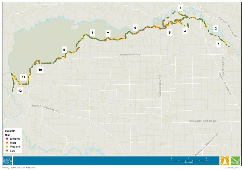
Figure 4-3 Points of weakness risk mapping for the Murray River levees. (Due to the scale of mapping, points overlap with the highest risk taking precedence)
